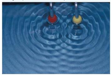
FIGURE 8.25 Nodal and antinodal lines in a ripple tank with two sources
