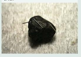
When molten ferromagnetic materials in lava cool down, the magnetic domains within the material are aligned by Earth's magnetic field, which form natural permanent magnets.
