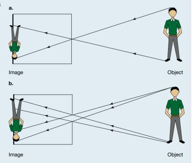
The size of this image depends on the distance of the pinhole from the object: the closer the object, the larger the image. The size of this image also depends on the size of the box: the longer the distance from the pinhole to the screen, the larger the image.
