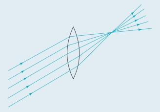
Placing a lens at the large pinhole that focuses that light onto a point on the screen enables the clear image to be produced, as shown in figure 11.9.5.
