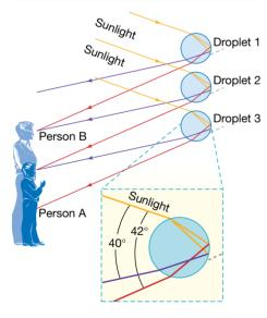
FIGURE 2.27 A light ray enters the bottom of the raindrop, is reflected twice off the wall of the raindrop, then emerges.
