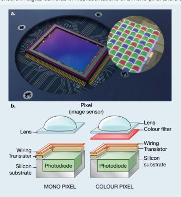
Pixels convert light energy into electrical energy and store it in the pixel. A reader measures the electrical energy stored in each pixel one by one. The combined measurements are processed, and the photo is stored as a digital image binary code.
