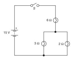
a. Determine the equivalent resistance of the circuit.
