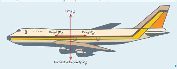
In figure 11.3.9, all the forces are modelled as acting at the centre of gravity; however, lift and drag can be modelled more accurately as acting at the centre of pressure. When viewing an aircraft from the side, the centre of pressure is approximately in the middle of the wings, which is slightly closer to the rear of the plane than the centre of gravity. The centre of pressure is important to consider when analysing how the forces and torques affect the stability of an aircraft.
