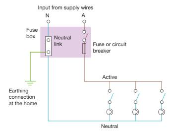
In power circuits, a third wire is used. This is called the **earth wire**. It connects the case of the appliance being used to the earth as a safety device. Its function is discussed in section 7.3.8. Otherwise, a power circuit operates in exactly the same way as a lighting circuit, with the current oscillating between the active and neutral wires through the appliance. Figure 7.5 shows how three-point power
