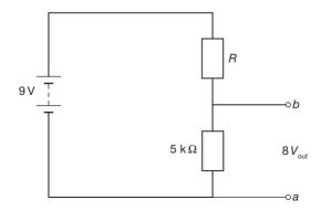
a. Determine the value of the unknown resistor.
