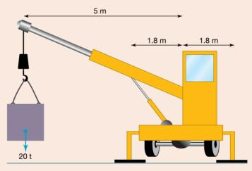
If the mass of the truck is evenly distributed, how heavy must the truck be if it is not to tip over?
