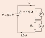
5. MC The following circuit diagram shows a voltage divider.
