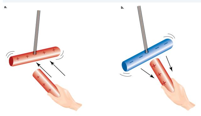
It was quickly observed that like-charged objects repelled each other while unlike-charged objects attracted each other. Charged objects exert a force on each other. The force between two stationary charged objects is called an electrostatic force.
