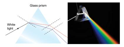
As light enters a triangular glass prism, it is refracted towards the normal. It then travels through the prism to the other side, where it is refracted away from the normal, because the light is re-emerging into the air.
