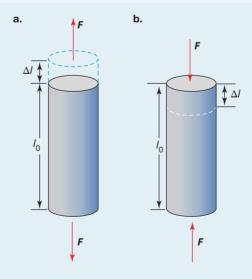
Analyse the behaviour of materials under load in terms of extension and compression, including Young's modulus,  $E = \sigma/\varepsilon$ , area under stress versus strain graphs and the elastic or plastic behaviour of materials under load
