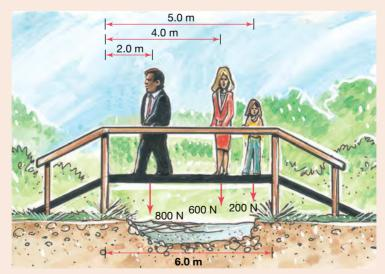
Calculate the reaction at each end when the three people are in the positions shown.
