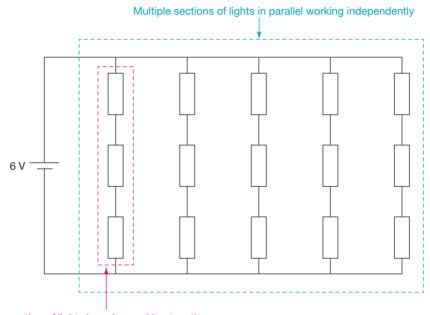
One section of lights in series working together
