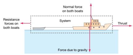
dinghy, it will move with a constant velocity. If the tension in the rope is less than the resistance forces on the dinghy, it will slow down; that is, its acceleration will be negative.
