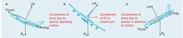
For a plane to undertake level flight at a constant velocity, torques must be balanced in addition to the forces being balanced to ensure rotational stability. Recall from subtopic 9.8 that torque is calculated as force multiplied by the perpendicular distance between the force and pivot.
