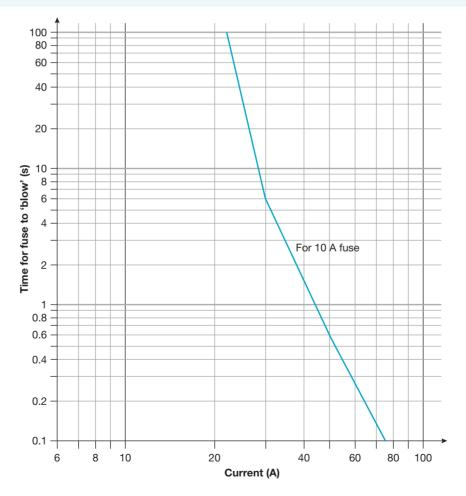
If the current is flowing through a person to the earth, the following principles should be followed: the current should be as small as possible and the time of exposure to the current should be as short as possible. Fuses are not designed to meet these requirements. Their main function is to prevent fires in buildings due to the overheating of wires when they carry too great a current.
