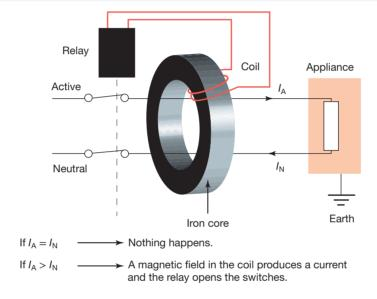
However, if there is an electrical fault and a residual current flows to the earth via the earth wire or a person, the current in the active wire will be greater than in the neutral wire. The residual current is the difference between the active and neutral currents. The magnetic effects of the two currents will no longer cancel. A current is then produced in the relay circuit, and both the active and neutral wires of the circuit are broken by a switch.
