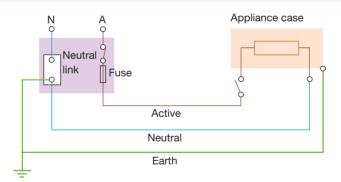
Note that in both the lighting and power circuits the switch is in the wire connecting the device to the active wire. A switch in the neutral wire would also turn off the device, but the functional parts of the device — such as the element of a toaster — would still be directly attached to the active wire and would be 'live'.
