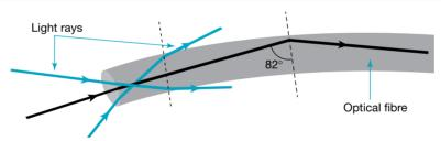
If the glass fibre is exposed to the air, the critical angle for light travelling from glass to air is 42°, which is quite small. Any angle of incidence greater than this angle will produce total internal reflection. If the fibre is very narrow, this angle is easily achieved.
