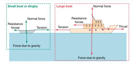
Figure 9.23 shows only the forces acting on the whole system of the two boats and the rope joining them. When Newton's Second Law is applied to the whole system, the system is considered to be a single object.
