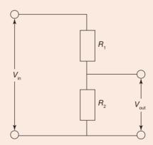
MC If  $V_{\rm in} = 12$  V,  $R_1 = X$ ,  $R_2 = 50$   $\Omega$  and  $V_{\rm out} = 7.5$  V, what is the resistance X?
