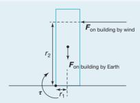
Calculate the stress and strain resulting from the application of compressive and tensile forces and loads to materials in structures,  $\sigma = F/A$ ,  $\varepsilon = \Delta l/l$
