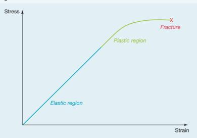
Similar to force—displacement graphs for a spring, the area under a stress—strain graph gives the amount of energy absorbed by a material. Note that a material will typically exhibit different stress—strain behaviours depending on whether it is experiencing compression or tension loads.
