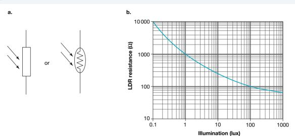
Note: A logarithmic scale is a non-linear scale and is commonly used as an effective way of displaying data that cover a large range of values on one graph. By plotting the log of resistance and the log of illumination, we are able to graphically plot two parameters.
