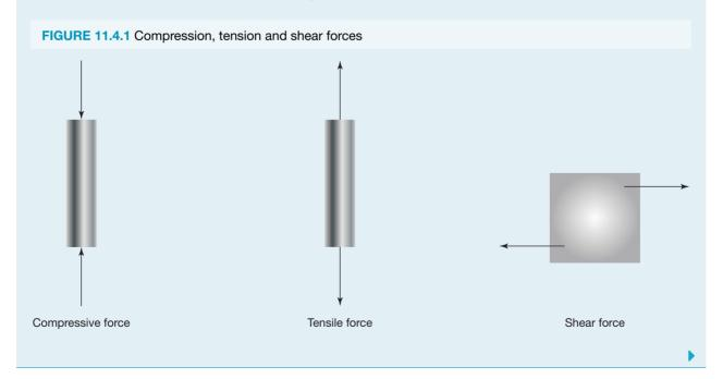
Structures often need to withstand all three types of forces. The bridge shown in figure 11.4.2 is subjected to the load from the weight of the truck. Forces act at each abutment in accordance with Newton's Third Law to balance the load. Shear forces are experienced by the bridge deck between the truck and each abutment.
