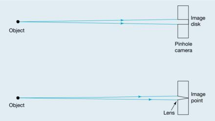
Simple cameras, like many small 'point and shoot' cameras and those in mobile phones, use a very small opening called an *aperture*, which allows light to pass to the film or sensor so that the camera does not need to change focus for each photo taken. They have a large depth of field but do not function well in low-light environments or when the objects are moving quickly.
