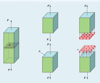
To avoid failure, materials used in structures must be able to withstand stresses generated by compression, tension and shear forces, examples of which are shown in figure 11.4.7.
