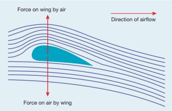
As you can imagine, the force applied on the air by the wing does not act perfectly vertically, resulting in a horizontal force component in addition to the vertical force component. The same is also true for the force on the wings by the air, as shown in figure 11.3.8. It is the vertical component, the force on the wings by the air,  $(F_y)$ , that we call lift.
