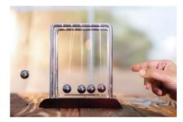
Vicki wanted to take this investigation further and determine how the size of the balls affected the time for movement to stop.
