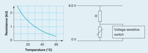
As the temperature drops, the resistance of the thermistor increases. As the thermistor's resistance increases, its share of the voltage from the power supply also increases, while that of the fixed value resistor will decrease.
