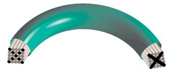
FIGURE 2.18 A light ray travels along an optical fibre through total internal reflection.
