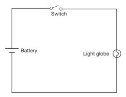
A battery is connected to a light globe and a switch. The emf of the battery is 4.2 V. The switch is currently open.
