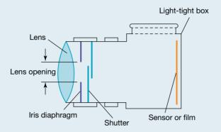
The functional parts of a basic film camera are illustrated in figure 11.9.12.
