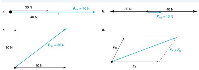
Note that in more complex cases, it is far easier to list the x and y components of each vector, sum the x components and sum the y components, and then use Pythagoras' theorem to calculate the resultant force.
