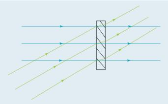
If we grind the glass block down so that it is now shaped like the one in figure 11.9.3, refraction converges (bends the rays to meet at a point) the three rays in each case. This works for these three rays from the two angles, but if we grind the lens so that it is a continuous curve in the arc of a circle (or better, a parabola), we find that the convergence occurs for all sets of parallel rays that hit the lens, as shown in figure 11.9.4.
