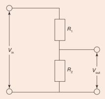
If this case,  $V_{\rm in}$  = 9.0 V,  $R_{\rm 1}$  = 40  $\Omega$  and  $R_{\rm 2}$  = 60  $\Omega$ .
