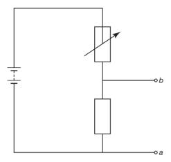
What happens to the voltage drop  $V_{\rm ab}$ , when the resistance of the variable resistor decreases and the other resistance is unchanged? (1 mark)
