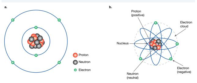
Protons and electrons possess a characteristic known as electric charge; because of their electric charge, these particles exert electric force on each other. Protons carry a positive charge and electrons carry a negative charge. The positive charge on a proton is equal in magnitude to the negative charge on an electron, meaning that the negative and positive charges are balanced and can **neutralise** each other. Neutrons have no electric charge; that is, they are uncharged or neutral.
