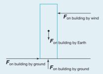
2. Rotational equilibrium: the ground must be able to generate a torque that is equal and opposite to the torque generated about the bottom left corner of the building. Note that the clockwise torque generated by the weight of the building helps to balance the anticlockwise torque generated by the force of the wind.
