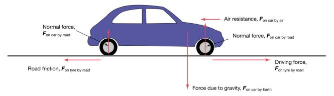
The net force acting on the car in figure 9.19 is zero. It is therefore moving along the road at constant speed. We know that it is moving to the right because both the air resistance and road friction act in a direction opposite to that of motion. If the car were stationary, neither of these forces would be acting at all.
