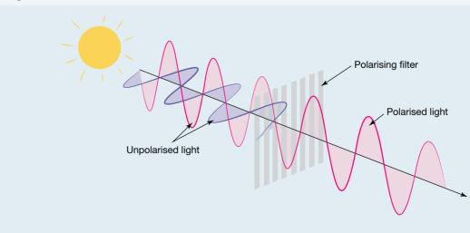
FIGURE 11.9.18 An example of the effect of a polarising filter (used for the photograph on the right)
