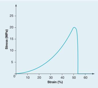
Similar to the force—displacement graph for a spring, the area under a stress—strain graph gives the amount of energy absorbed by a material. The term 'toughness' is used to describe the ability of a material to store energy up to the point of failure. A material with a greater strain energy up to fracture is said to be tougher than one requiring less energy.
