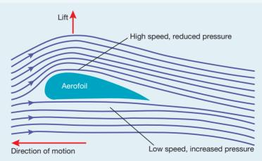
**FIGURE 11.3.6** The curved upper surface of an aerofoil forces air to travel more quickly over the top of the aerofoil than below it.
