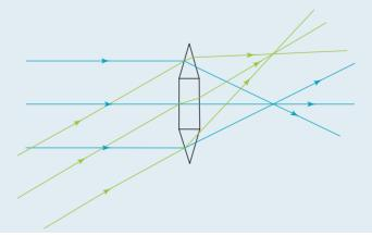
FIGURE 11.9.4 Refraction converges all rays when a lens is curved.
