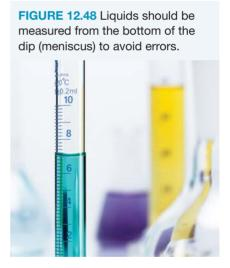
errors differences between a measurement taken and the true value that is expected; errors lead to a reduction in the accuracy of an investigation
