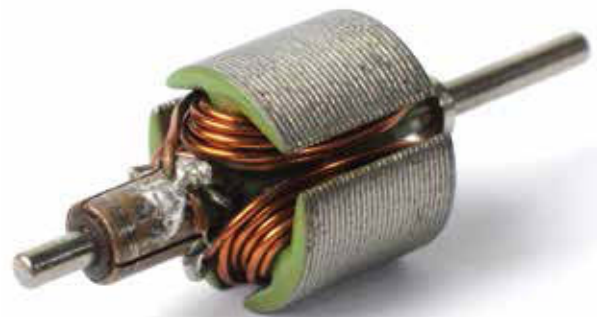
Commutator and coil from a hair dryer
