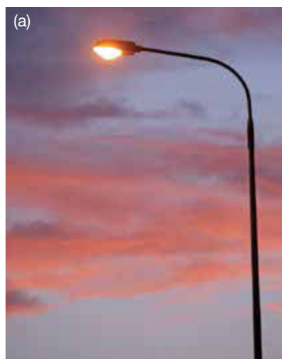
(a) Sodium vapour street light (whose spectrum is dominated by its yellow emission lines), (b) characteristic colour of sodium flame, (c) visible line spectrum of sodium atoms, and (d) visible line spectrum of hydrogen atoms
