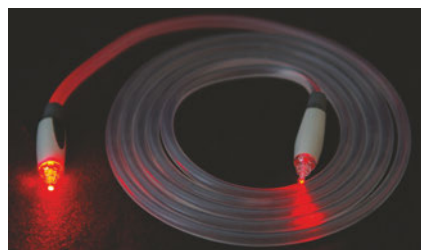
Figure 5 Total internal reflection in a glass rod and the use of total internal reflection to transfer a light signal from one end of an optical fibre to another
