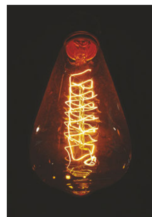
Figure 4 The heated tungsten filament of an incandescent globe
