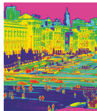
Figure 3 A thermal image. Redder colours indicate higher temperatures.
