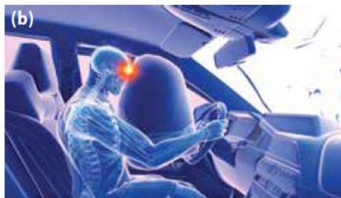
Figure 6 (a) A car crash without an airbag will result in a large force on the driver as the impulse occurs over a short duration. (b) An airbag acts to slow the collision and reduce the amount of force experienced by the driver.
