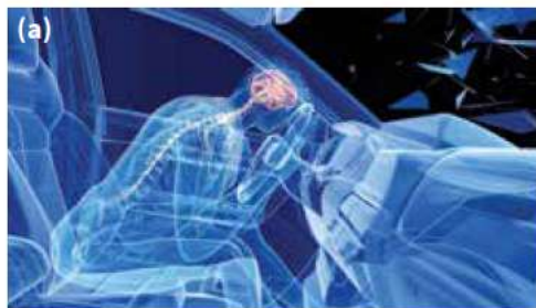
Figure 6 (a) A car crash without an airbag will result in a large force on the driver as the impulse occurs over a short duration. (b) An airbag acts to slow the collision and reduce the amount of force experienced by the driver.
