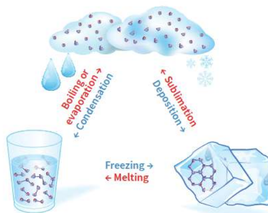
Figure 4 The transitions between states of matter. Energy must be absorbed by the substance for the processes with red arrows. Energy is released by the substance for the processes with blue arrows.
