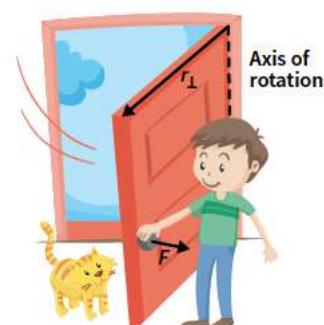
Figure 2 A door experiences torque when a force, F , acts perpendicular to the door at a distance, r_{\perp} , from the hinges.
