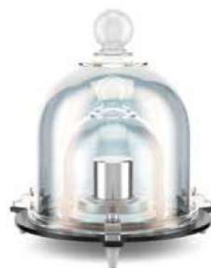
Figure 1 A 3D rendering of the IPK (International Prototype of the Kilogram). The kilogram was the last unit to be defined in terms of a physical object. Prior to 2019, it was defined by the mass of the IPK, a cylinder made of platinum and iridium that was kept in a vault in France.
