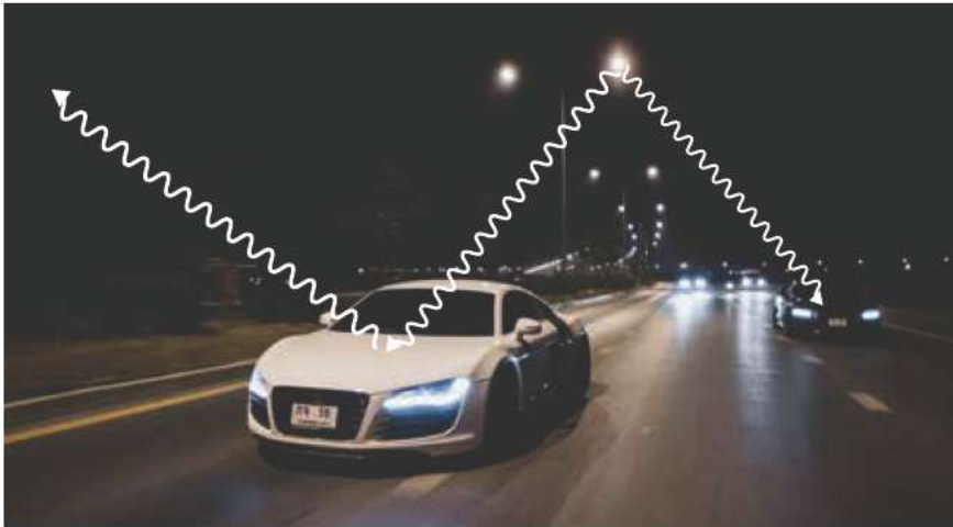
Figure 1 For a light coloured surface, most of the incoming (visible) radiation is reflected, which we see, but for a dark coloured surface, most of the incoming (visible) radiation is absorbed rather than reflected.
