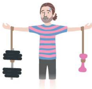
Figure 11 The torque on a body will be larger when a greater force is applied at the same radial distance.
