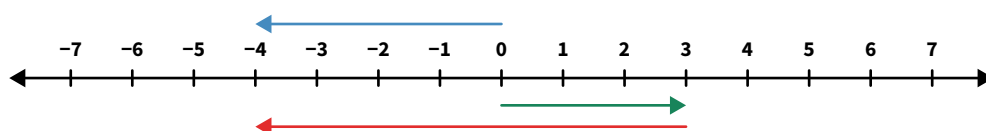
Figure 2 We now have one of the vectors pointing in the positive direction and one in the negative. We can still combine these two vectors together, with the net effect of this combination shown by the blue arrow.
