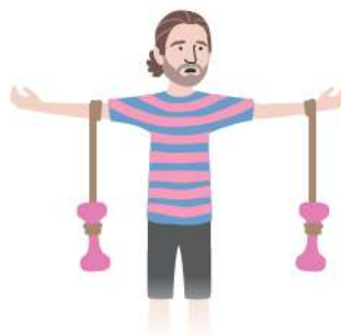
Figure 12 The torque on a body will be larger when the distance to the pivot point is larger.
