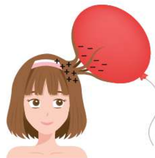
Figure 3 The action of rubbing a balloon on hair transfers electrons from the hair to the balloon.
