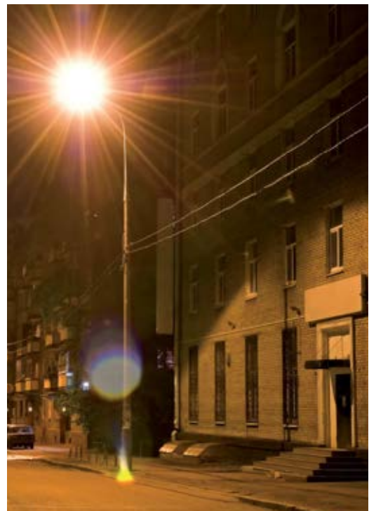
Figure 15.10 Street light trespassing into windows
