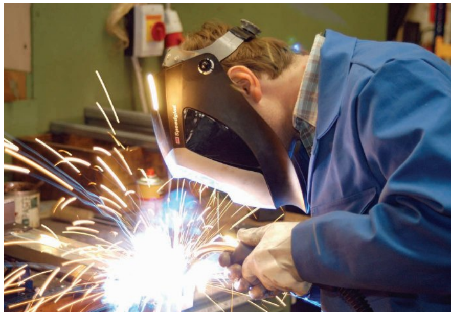
Figure 9.3 An auto-darkening helmet is worn by a welder.
