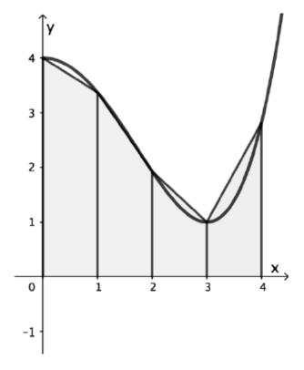
Using the trapezium rule, the approximate area calculated is equal to
