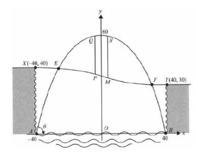
The main frame of the bridge has the shape of a parabola. The parabolic frame is modelled by  $y=60-\frac{3}{80}x^2$  and is connected to concrete pads at B(40,0) and A(-40,0). The road across the gorge is modelled by a cubic polynomial function.
