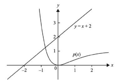
The line y=x+2 and the tangent to the graph of p at x=a intersect with an acute angle of heta between them.
