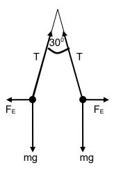
Just considering the left-hand side for all the forces to be balanced, T needs to be resolved into two components, one vertical and the other horizontal.
