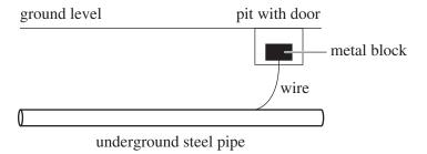
The metal block in the diagram is commonly magnesium, zinc or aluminium.
