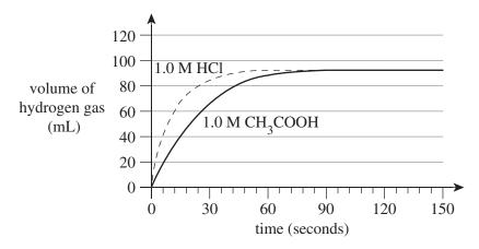
At the end of the experiment, no magnesium ribbon remained in the test tubes.
