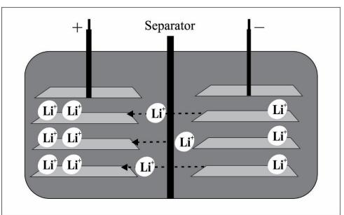
Since the discharge reaction is  $\text{Li}_x\text{C}_6(s) + \text{Li}_{1-x}\text{MnO}_2(s) \to \text{C}_6(s) + \text{LiMnO}_2(s)$ , the discharging half-equations involve the conversion of  $\text{LiC}_6$  to  $\text{C}_6$  and the conversion of  $\text{Li}_{1-x}\text{MnO}_2$  to  $\text{LiMnO}_2$ . This suggests that  $\text{Li}^+$  is released at one electrode and  $\text{Li}^+$  is gained at the other electrode, which is consistent with the discharging half-equations.
