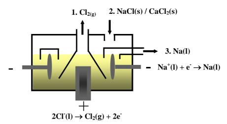
In the Down's cell, **gaseous Cl<sub>2</sub>** comes off the anode and **molten Na** is collected at the cathode. A mixture of NaCl and  $CaCl_2$  is fed into the cell where it liquefies. The  $CaCl_2$  serves to lower the melting temperature of NaCl.
