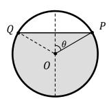
Area of the sector subtended by the angle  $\angle POQ$  is given by  $\frac{2\theta}{2\pi}\pi r^2 = \theta$  [1/2]. The area of the triangle  $\triangle POQ$  is given by  $\sin \theta \times \cos \theta = \frac{1}{2}\sin 2\theta$  [1/2]. So the area of the unshaded segment is given by  $\theta - \frac{1}{2}\sin(2\theta)m^2$  [1]
