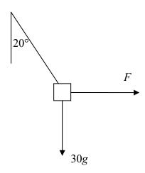
The magnitude of the horizontal force, F newtons, required to hold a 30 kilogram child in equilibrium on a swinging rope, as shown in the diagram above, is
