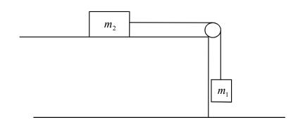
Two particles of mass  $m_1$  and  $m_2$  are connected by a light string that passes over a smooth pulley. The particle of mass  $m_2$  is at the point of moving over the rough horizontal table. The normal force is N and the tension force in the string is T. The coefficient of friction is
