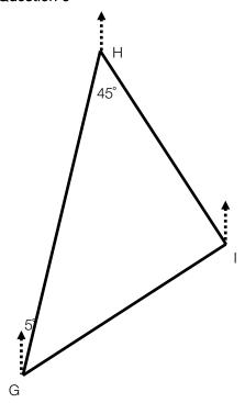
The bearing of point H from point G is 005° and the angle GHI in the triangle GHI is 45°. The diagram above shows this situation.
