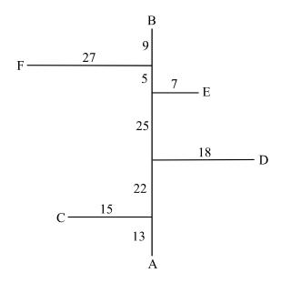
The diagram above shows a field sketch from a traverse survey with a base line AB. The distances in metres along AB between the perpendicular offsets are given as are the distances from the base line to the features at points C, D, E and F. The straight line distance between point A and point E in metres is closest to
