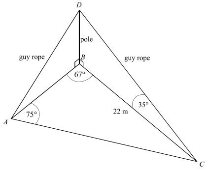
Two guy ropes AD and CD are attached to the top of a vertical pole BD and are anchored to the ground at points A and C respectively. Points A, B and C lie in a horizontal plane. In triangle ABC,  $\angle BAC = 75^{\circ}$ ,  $\angle ABC = 67^{\circ}$  and BC = 22 metres.
