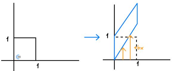
Shear of a factor b parallel to the y-axis.
