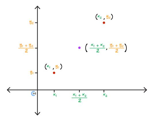
The midpoint, M, of two points A and B is simply the point halfway between A and B.
