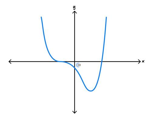
E.g.,  $f(x) = (x - a)^3 (x - b)$  has an x-intercept (a, 0) which is also a stationary point of inflection.
