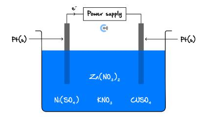
**a.** State and explain what metal will accumulate on the cathode immediately when the power supply is turned on. (2 marks)
