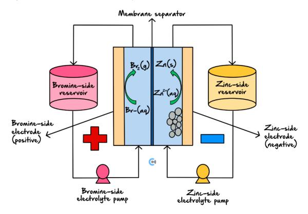
It can both discharge and recharge. The reactions that occur within the cell are shown below:
