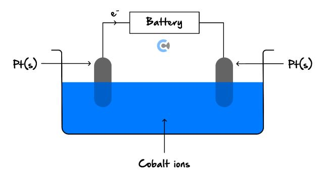
Kynan runs the cell for 20.0 minutes with 5.50 A running through the cell and finds that 2.0 g of metal has been deposited on the cathode.
