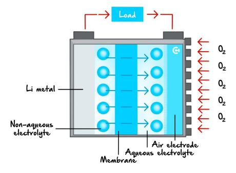
The following reaction occurs in an acidic electrolyte whilst the cell is undergoing discharge:
