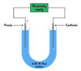
Several drops of phenol red were added to the solution next to each electrode.
