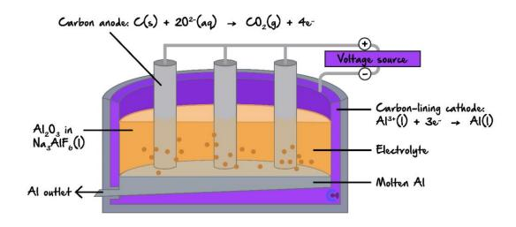
**a.** If the cell is typically enclosed, explain why it is necessary to include a gas pump that is separate from the Al outlet. (2 marks)
