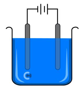
**NOTE:** Even though solid copper (Cu(s)) is the strongest reductant in this scenario, it is at the cathode which is the wrong electrode, and thus it cannot oxidise.
