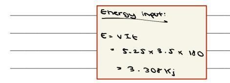
ii. Calculate the total energy absorbed by the calorimeter.
