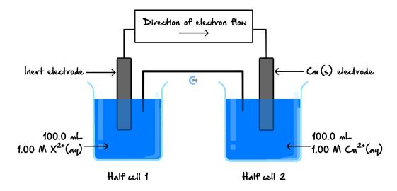
After discharging 2654 C of electricity, the concentration of the  $X^{2+}$  (aq) in solution in half cell 1 was found to be 0.725 M. The volume of the solutions in the two half cells had not changed.
