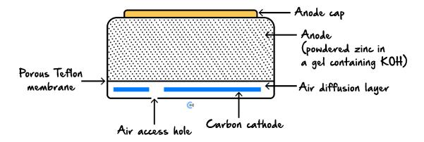
The zinc acts as the anode. It is in the form of a powder dispersed in a gel (a jelly-like substance) that also contains potassium hydroxide. The cathode consists of a carbon disc. Oxygen enters the cell via a porous Teflon membrane. This membrane also prevents any chemicals from leaking out.
