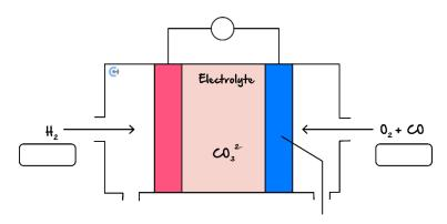
In this MCFC, hydrogen is being used as a reactant alongside  $O_2(g)$  in order to produce energy. The main carbon-containing product of the cell is carbon monoxide.
