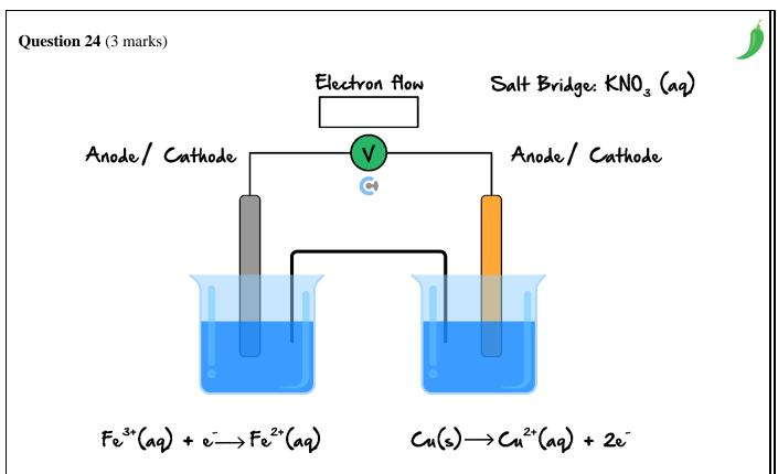
Use the provided diagram of a galvanic cell, and label the cathode, anode, electron flow and ion movement in the salt bridge.
