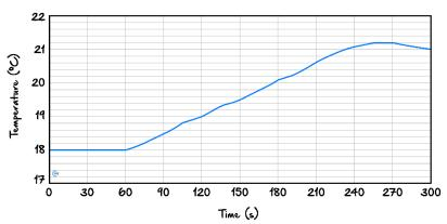
The calorimeter was calibrated using a current of 2.7 A, starting at 60 s. The current was applied for 180 s and the applied voltage was 5.4 V.
