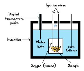
A 1.50 g sample of air-popped popcorn is placed in the bomb calorimeter. The initial temperature of the water is 22.2°C and the final temperature is 25.7°C. Assume that the air-popped popcorn is fully combusted. The calibration factor for the bomb calorimeter is 6.54 kJ °C<sup>-1</sup>.
