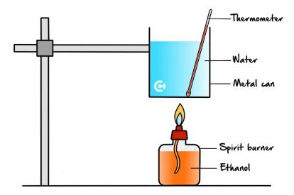
They wanted to calibrate the set up first through combusting ethanol. The spirit burner intially weighed 25.0 g. It then underwent complete combustion and the weight of the spirit burner was recorded to be 21.8 g. The beaker contained 300 g of water and increased in by 35.70 °C.
