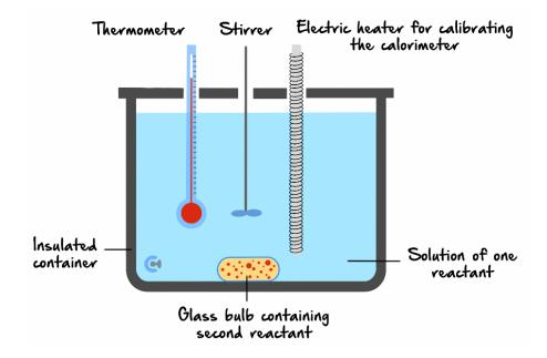
Which of the following correctly outlines the main purpose of the glass bulb?
