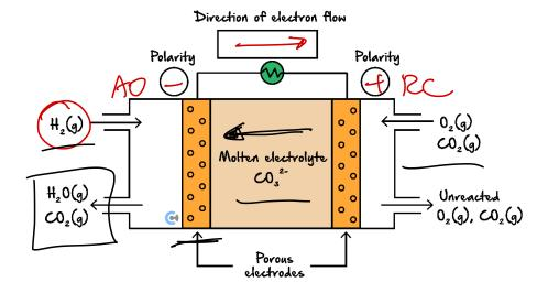
At one electrode of the MCFC, carbon dioxide,  $CO_2$ , gas reacts with oxygen,  $O_2$ , gas to form carbonate ions. At the other electrode, hydrogen,  $H_2$ , gas reacts with molten carbonate ions to form steam and  $CO_2$  gas.
