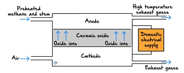
i. Write an equation for the reaction at the cathode where atmospheric oxygen is converted to oxide ions.(1 mark)
