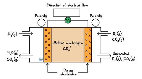
At one electrode of the MCFC, carbon dioxide,  $CO_2$ , gas reacts with oxygen,  $O_2$ , gas to form carbonate ions. At the other electrode, hydrogen,  $H_2$ , gas reacts with molten carbonate ions to form steam and  $CO_2$  gas.
