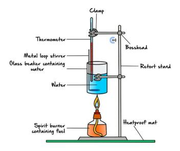
He burns the fuel, heating the 301.5 mL of water from 17.0°C to 64.0°C, leaving a spirit burner with a mass of 221.10 g.
