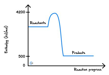
i. Given that the activation energy for this reaction is  $+400 \ kJ/mol$ , find the change in enthalpy ( $\Delta H$ ) for the reverse reaction. (1 mark)
