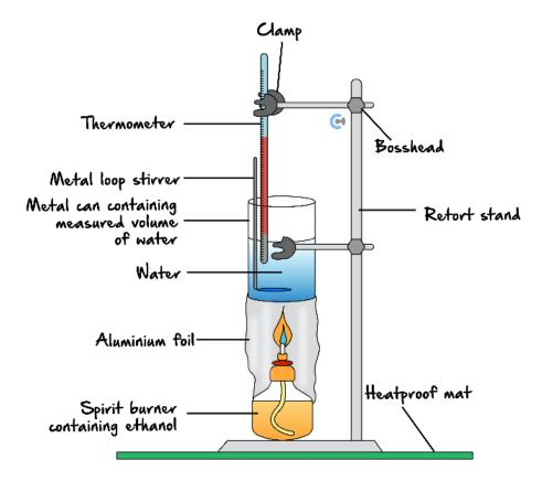
Atharva wants to increase how precise their results are and decides to use aluminium foil and wrap the opening between the flame and the beaker of water as shown above.
