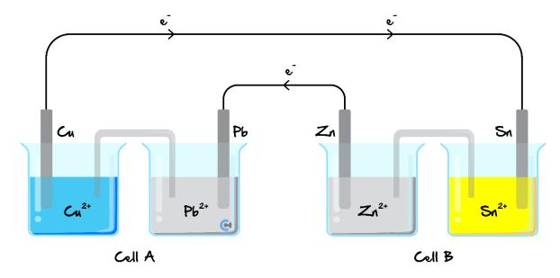
**a.** Identify if each of cell A and cell B act as galvanic or electrolytic cells. (1 mark)
