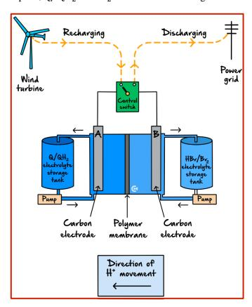
During discharge, QH<sub>2</sub> is converted to Q and Br<sub>2</sub> is converted to HBr.
