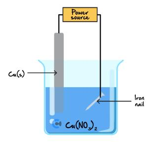
**a.** Explain which terminal of the power source the nail should be connected to and why. (2 marks)
