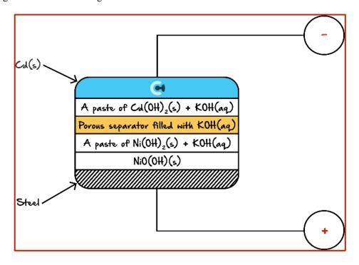
The overall cell reaction for the cell when discharging is:
