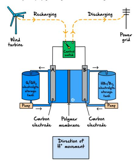
During discharge, QH<sub>2</sub> is converted to Q and Br<sub>2</sub> is converted to HBr.
