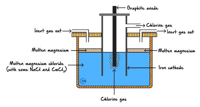
The design of this cell takes into account the following properties of both magnesium metal and magnesium chloride:
