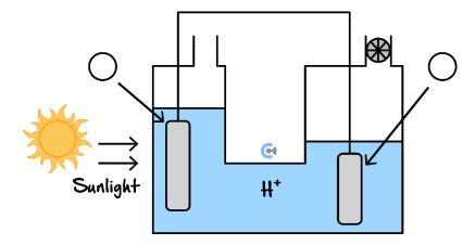
**a.** Given that the sunlight causes the oxidation of water, label the polarities of the electrodes by placing a + or – sign in the circles above. (1 mark)
