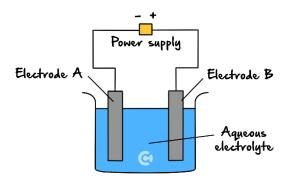
After the current had passed through the cell for some time, a reddish brown liquid was formed at the electrode B, while a metal was found deposited on the electrode A.
