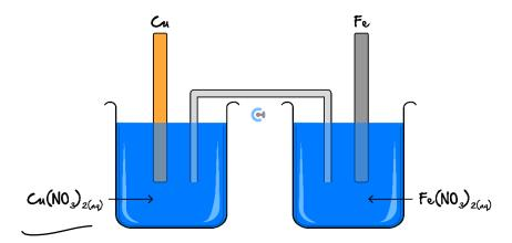
The solutions are connected to each other with a salt bridge consisting of an inverted U-tube containing an appropriate electrolyte.
