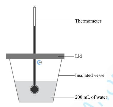
The amount of water present in the calorimeter is increased to  $250 \ mL$ , changing the calibration factor.
